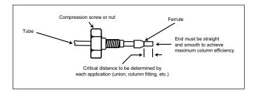
Figure 1. Ferrule and compression screw assembly
