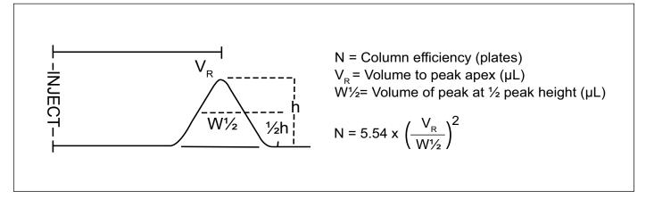
Figure 2. Half height method test calculations
