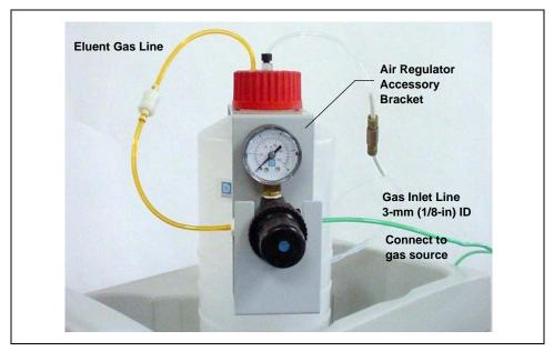
Figure 46. ICS-1000 Pressurized Eluent Reservoir Connections (Optional)
