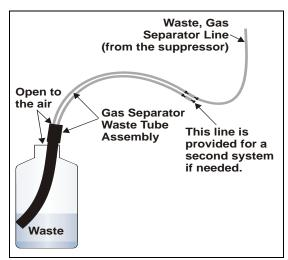
Figure 22. Gas Separator Waste Tube Installation
