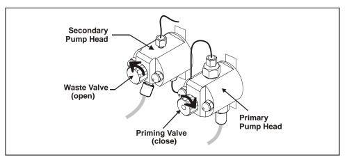
Figure 37. Priming the Pump
