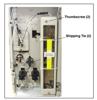
Figure 18. ICS-1000 Column Heater Setup
