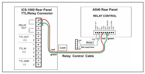
Figure 44. Example AS40 Autosampler Connection
