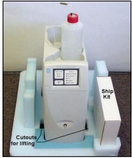
3. Remove the next layer of foam and remove the Ship Kit box (see Figure 3).
