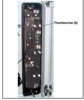
Figure 19. ICS-1000 Column Heater Cover Removed
