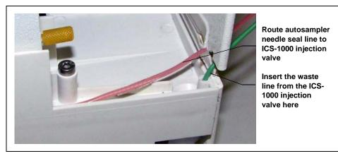
Figure 38. Autosampler Drip Tray
