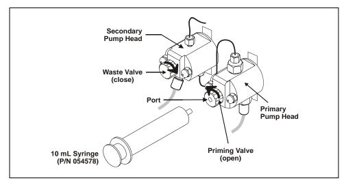
Figure 35. Priming the Eluent Lines
