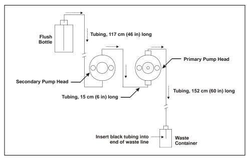
Figure 48. Piston Seal Wash Flow Schematic
