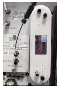
Figure 21. Suppressor Installed (SRS Shown)
