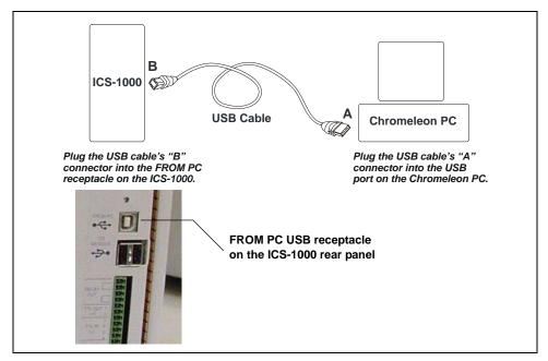
Figure 7. Example Connections: One ICS-1000 Connected to the Computer
