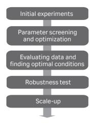
The robustness of a process is a measure of its capacity to remain unaffected by variations, and shows the process reliability during normal usage. A robustness test evaluates factors potentially causing variability in the process, detected by responses of methods, for example purity and yield. For this purpose, small deliberate variations in the process parameters are introduced.
