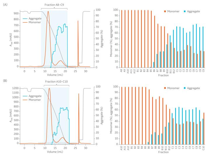
Fig 4. At a load of 66% of Q<sub>B10</sub> in 1 mL columns (10 cm bed height) with a flow velocity of 75 cm/h, (A) Capto Butyl ImpRes and (B) Butyl Sepharose High Performance both effectively decrease the aggregate content and show similar elution profiles.
