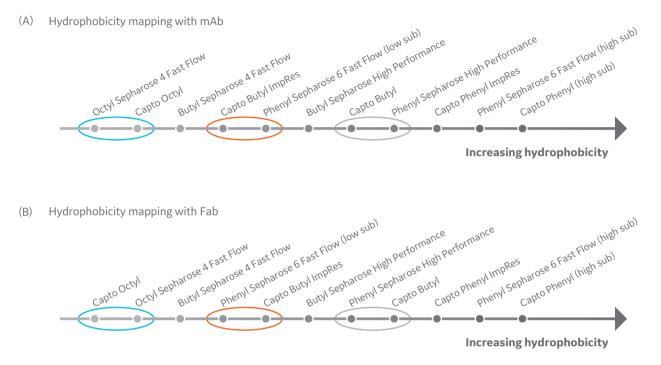
Fig 1 Hydrophobicity scale with a mAb and its corresponding Fab. Increasing hydrophobicity indicates increased binding strength and later elution in the gradient. The circles highlight where hydrophobicity order of the evaluated HIC resins is different between the studied molecules.
