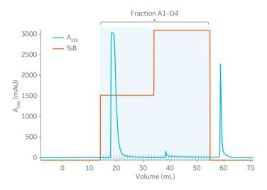
**Fig 6.** Results from Capto Butyl ImpRes with load of 65% of  $Q_{_{B10}}$  for mAb and aggregate mixture show favorable monomer yield with increased flow velocity (200 cm/h) and bed height (20 cm). From left to right, peaks represent the monomer, aggregate, and CIP. The marked fractions were analyzed for aggregate, see Figure 7.
