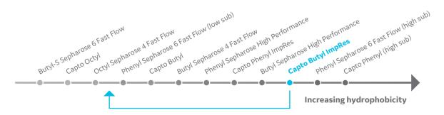
Fig 2 Hydrophobicity scale with model proteins from data file 29031925AB. The arrow highlights how hydrophobicity differs for Capto Butyl ImpRes with the mAb compared to different model proteins.
