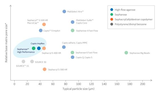
Fig 3. Capto Butyl ImpRes and Butyl Sepharose High Performance were chosen for the aggregate polishing step due to their small particle size and thus high-resolution properties. \*Relative base matrix pore size estimated by inverse size exclusion chromatography.
