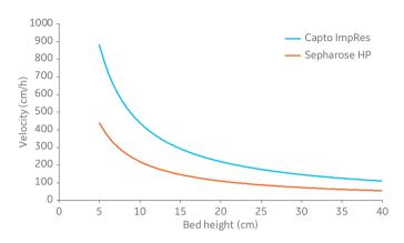
**Fig 5.** The window of operation (area below the curves) of Sepharose High Performance and Capto ImpRes resins. Data correspond to a process diameter column at 20°C and viscosity equivalent to water.
